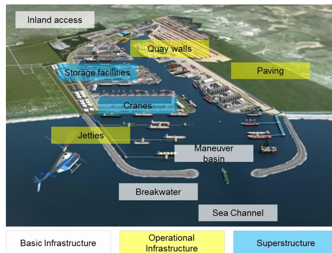
Figure 2: Port Infrastructure description
