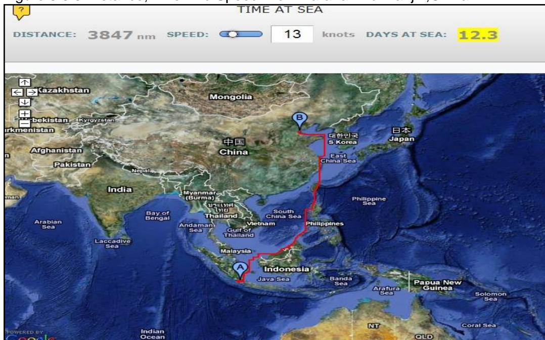
Figure 5.3.3 Distance, Time And Speed From Tarahan To Tianjin, China
