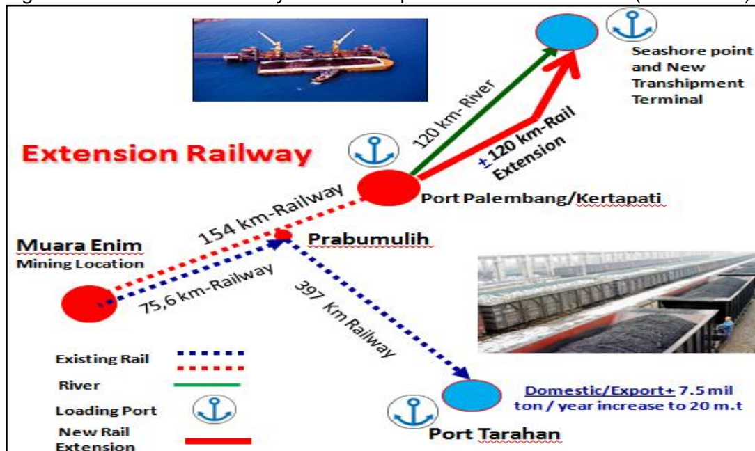
Figure 5.3.1 Extension Railway and Transshipment Scheme Networks (Scenario III)
