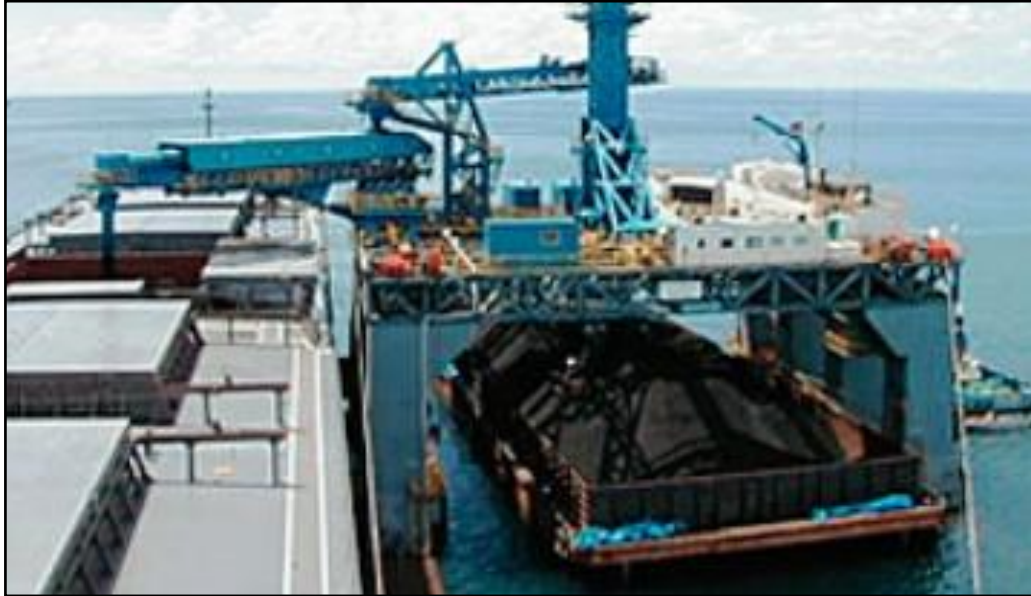
Figure 4.2.4 Semi Submersible Trans-shipper
