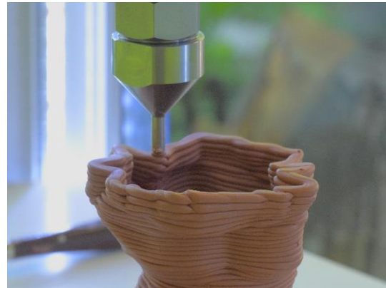
Figure 1: Clay printing process. Photo by Pauline Vaandrager, 2025
